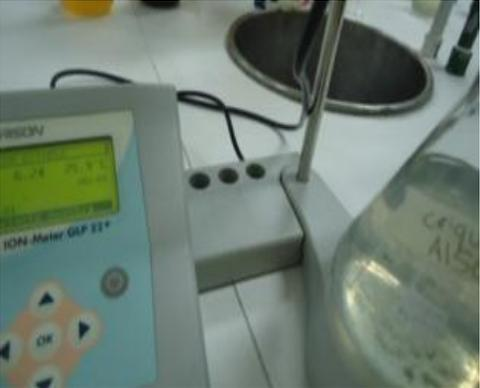
A photograph of a pH meter (ORION ION-Meter GMP 22+) with a glass electrode. The digital display shows a reading of 8.24. The electrode is submerged in a clear liquid in a beaker. |                                                                                                                                                                                                                                         |
