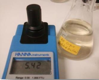
A photograph showing the same HANNA Instruments turbidity meter next to the beaker, which now contains a cloudy, turbid liquid. The meter's display shows a turbidity reading of 5.42 FTU. The beaker has a yellow label that reads 'H2O Cinc'. |
