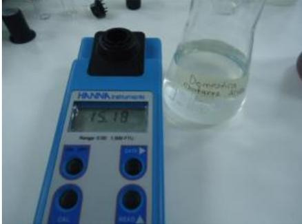
A photograph of a turbidity meter (HANNA HI9142) with a white sensor. The digital display shows a reading of 15.10. A beaker containing a clear liquid is next to it.             |                                                                                                                                                                                                                                         |
